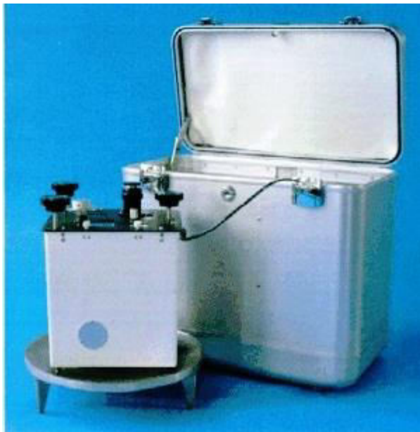
Figure (8): The LaCoste and Romberg gravimeter external shape and cross section showing its components.
