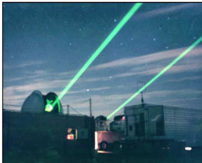
Figure (14): The process of tracking satellite by using the Transportable Laser Ranging System (TSLR) ground stations.
